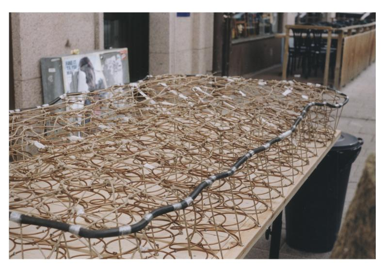
Found a tube I could fasten to the upper edge and around the springs. Chose the tube since the round bar didn't fit the round corners of the mattress. Bought a rubberised horsehair mat, cotton wool and three different types of fabric for the facing of the mattress.
