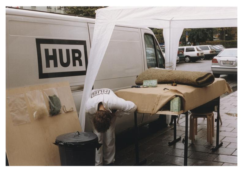
Fixed the thick woven fabric with tacks again and placed the rubberised horsehair mat on top, then two layers of cotton wool before facing it with a fabric made of cotton.
